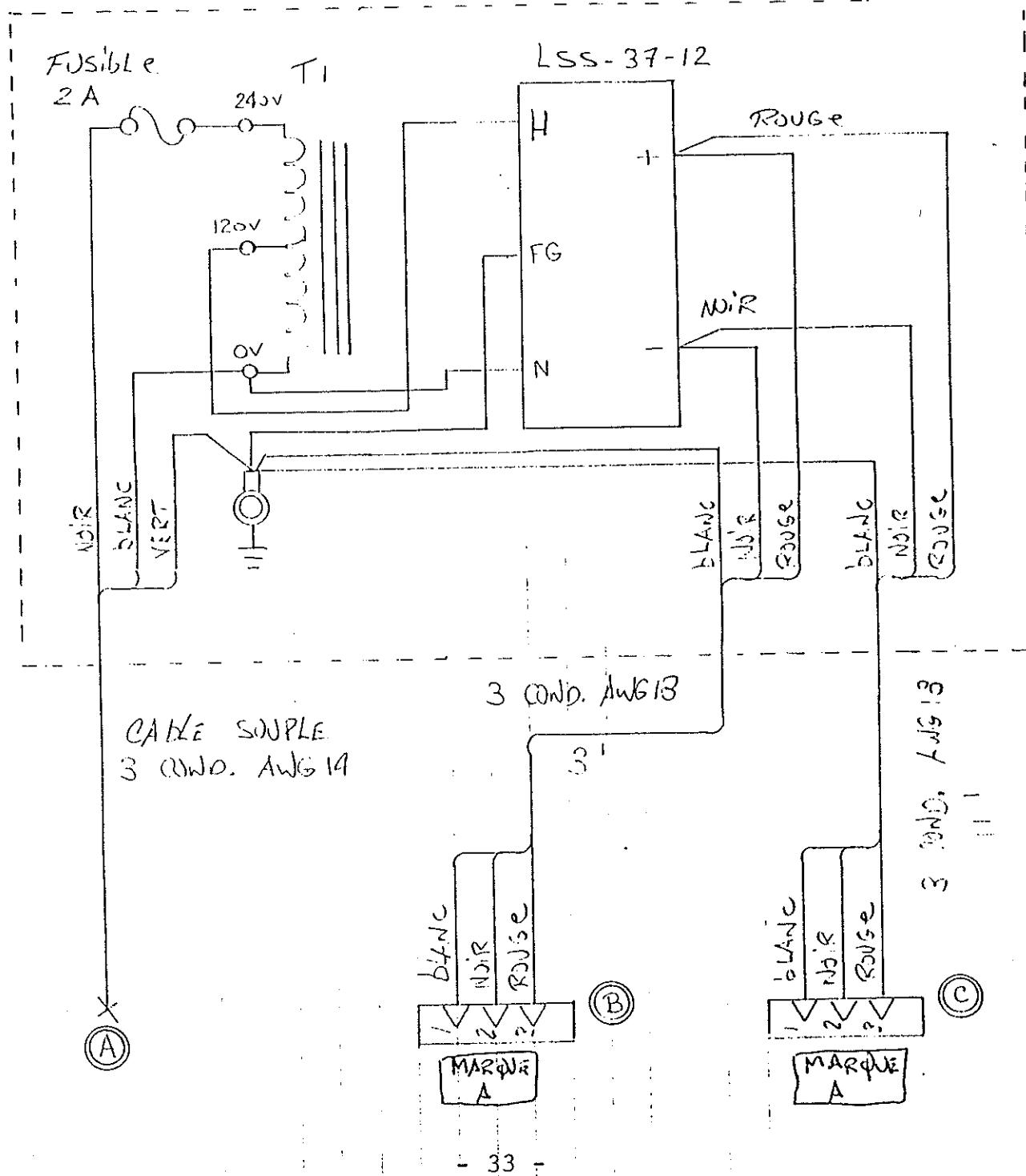
SCHÉMA DE DISPOSITION SYSTÈME ALIMENTATION
